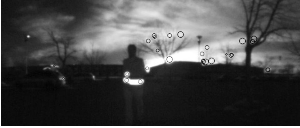
Figure 2.7: The figure illustrates the result of the feature detection process applied to an image I_f taken with IR flash. A reflective vest is visible in the center of the image. Detected features are drawn as black circles, the size of which indicates the feature scale s . The figure shows that under the influence of the IR light emitted by the sun, the feature set \mathcal{F}_{raw} includes many features that do not originate from a reflective vest.
