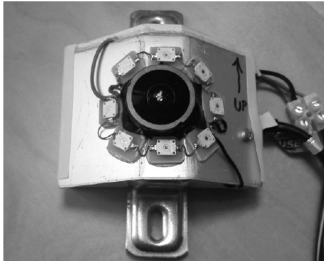
Figure 2.2: The single camera system used for image acquisition consists of a standard monochrome CMOS sensor, an infrared bandpass filter (not visible in the image), a fish-eye lens and a ring of 8 IR-LEDs.
