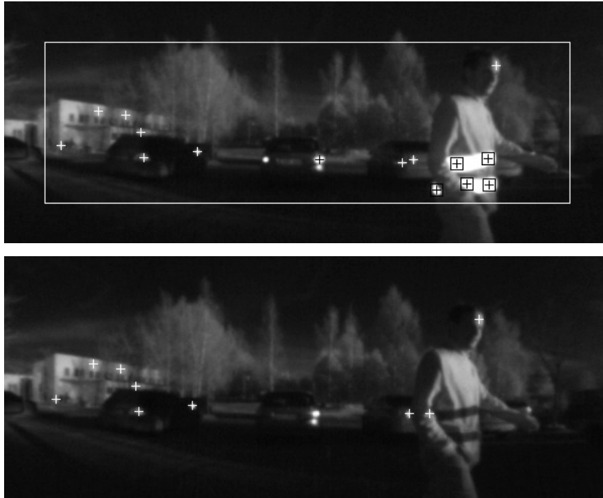
Fig. 3 The figure shows an exemplary result of the vest detection process. Blob-like features are detected in the image I_f taken with IR flash (above). Detected features are represented by the ensemble of crosses in I_f . The detected features are then tracked in the image I_{nf} taken without IR flash (below). The detection area in I_f is restricted to the white bounding box to allow features to be tracked even in the case of quick rotational movements. Successfully tracked features are marked as white crosses in image I_f and the tracked locations are indicated by white crosses in image I_{nf} . All tracked features in the above example show a very low intensity difference and are therefore not considered as vest candidates. Features that failed to be tracked include detections on the reflective vest as well as on the metallic surface of the car standing right in front of the camera. All the untracked features are considered as vest candidates and classified by the random forest model. A black square is drawn around features that are finally classified as vest features.
